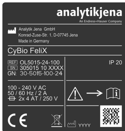
Fig. 7: Type plate for the version with enclosure/louver
